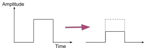
The effects of absorption can be reduced by using an **optical fibre repeater** to boost the signal at periodic positions along the fibre.
