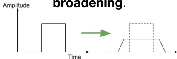
2. **Material dispersion** is a consequence of the signal containing several **different wavelengths**, each of which travels at slightly different speeds in the core. This again results in pulse broadening.
